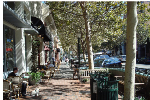
Figure 2 Wide streetsides, created by articulating building fronts and extending curbs, provide width for cafes and public spaces. Source: Kimley-Horn and Associates, Inc.
