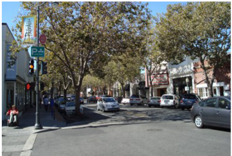
Figure 4 An example of alternating angled and parallel on-street parking on a main street. Source: Kimley-Horn and Associates, Inc.
